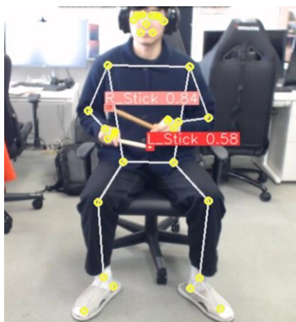
Figure 5: An example of real-time human posture tracking using the MediaPipe Pose Land-mark Model. The image shows the major landmark points of the entire body recognized by the machine learning algorithm.
