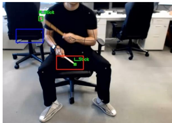
Figure 6: The image shows a system that tracks drumstick and body movements and generates drum sounds using the YOLOv8 model and MediaPipe's pose landmark model.
