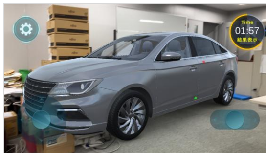
Figure 4: Gameplay interface displaying the virtual vehicle within the AR environment, with paint mottling defects (example: green sphere indicates correct identification, red sphere indicates user selection), timer, and viewpoint adjustment controls
